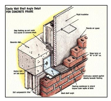
galvanized in case water leaks around the flashing.
