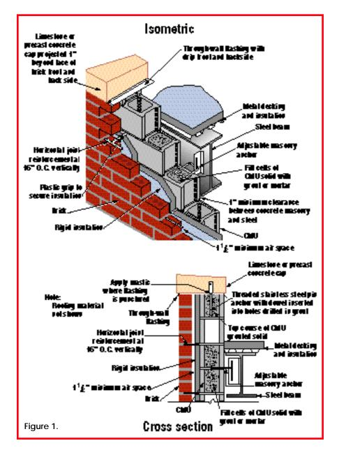
material with thermal properties similar to those of brick and concrete masonry, such as limestone, terra cotta, hard-fired clay, or precast concrete. Metal caps have a coefficient of expansion nearly three times greater than that of masonry, which leads to a significant amount of differential movement between the parapet cap and the wall below. If you use a metal cap, be sure to provide tightly sealed slippage joints where the cap sections lap.
